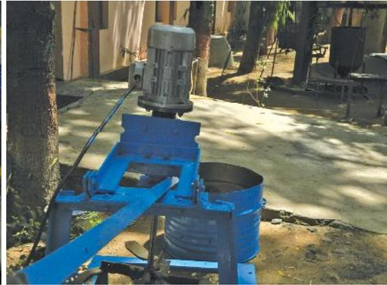
Custom soil puddling machine using 0.5 hp electrical motor
